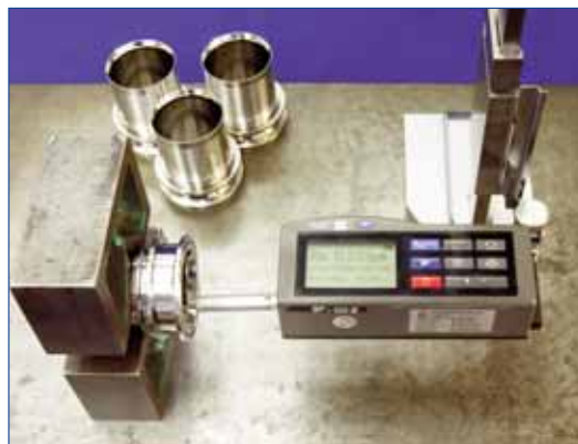
Surfscan, measuring internal surface finish
