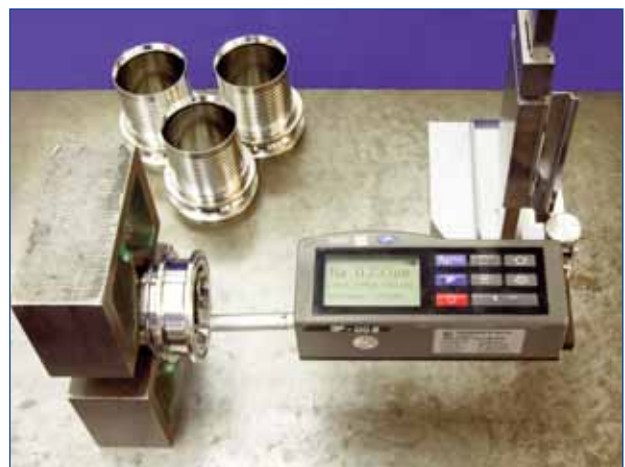
Surfscan, measuring internal surface finish
